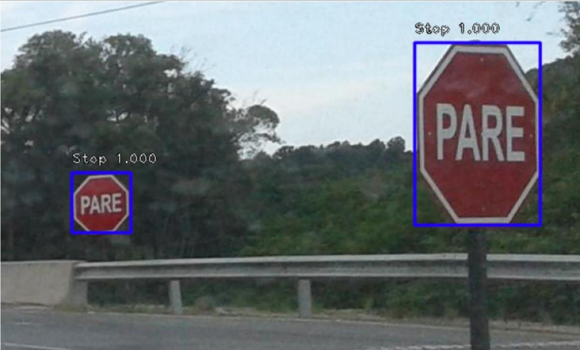
Figure 20: Detection and recognition of two Stop traffic signs within an image.
