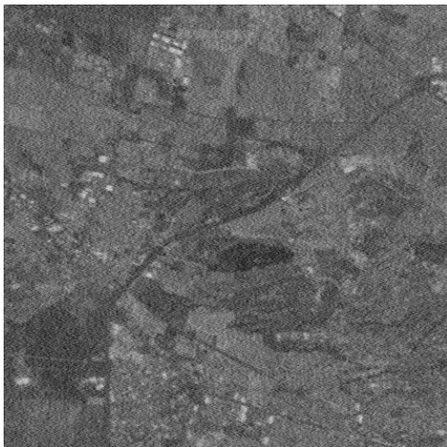
Fig. 3. Enhanced radar image formed applying the modified descriptive weighted constrained least squares (WCLS) algorithm.
