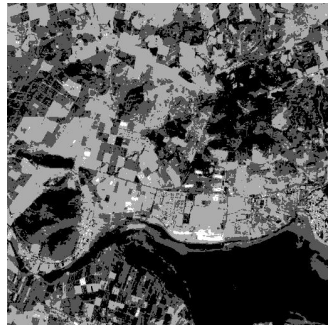
Figure 3. HEM extracted from the original high resolution SAR scene applying the MDM method.
