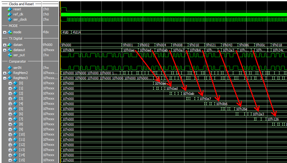
Figure 3.56 Operating Mode 14 – LFSR RXD Digital Loopback output signal saving waveform
