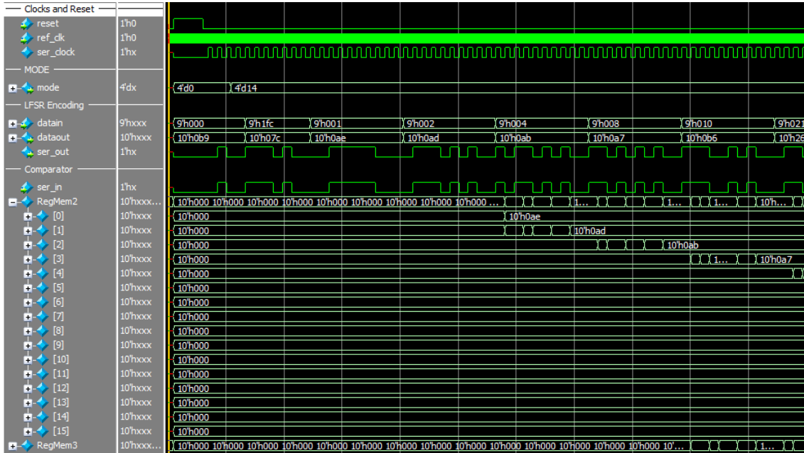
Figure 3.55 Operating Mode 14 – LFSR RXD Digital Loopback input signal saving waveform
