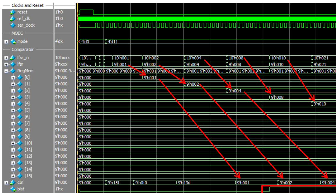
Figure 3.41 Operating Mode 11 – LFSR TXD Digital Loopback BIST waveform
