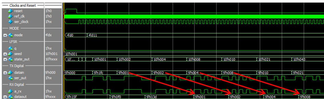
Figure 3.40 Operating Mode 11 – LFSR TXD Digital Loopback waveform
