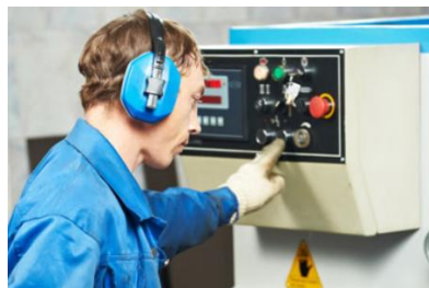
Figure 6. Old Human Machine Interface with buttons, switches, levels and light indicators.
