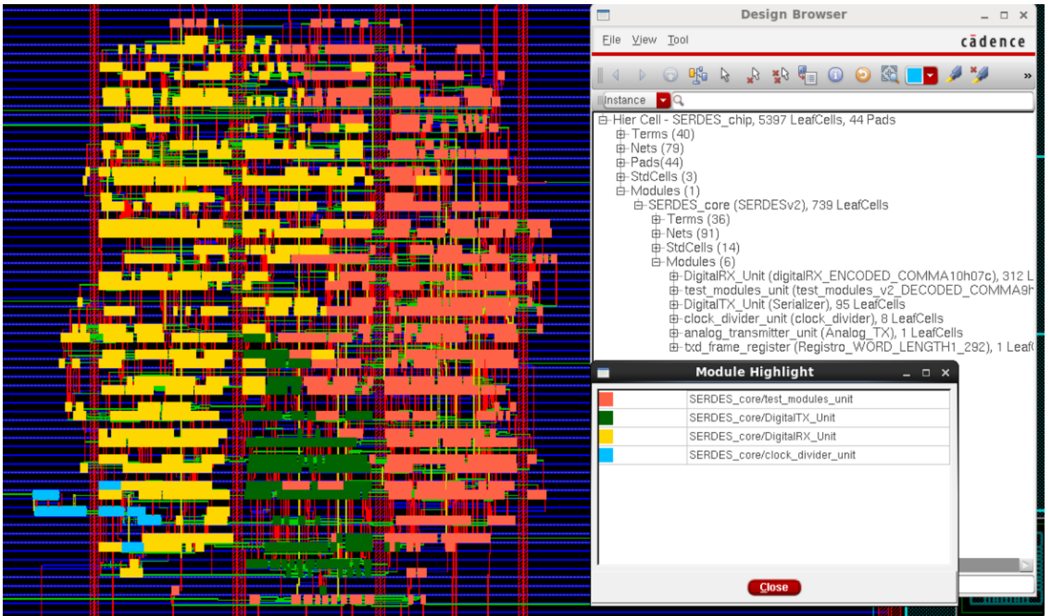
Figure 4.32. SerDes digital modules distribution in the layout.
