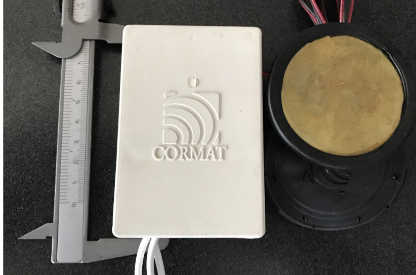
Fig. 2.12 Cabinet and wires with metal electrodes used for the RFD prototype.
