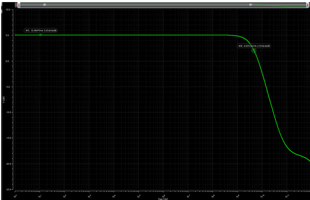
Fig. 3-15 Respuesta en frecuencia del OTA con W = 3.5 \text{ } [\mu\text{m}] , R_L = 1591.55 \text{ } [\Omega] , g_m = 1472.61 \text{ } [\mu\Omega^{-1}] , A_{v-sim} = 5.0542 \text{ } [\text{dB}] y BW_{sim} = 4.64 \text{ } [\text{GHz}] .
