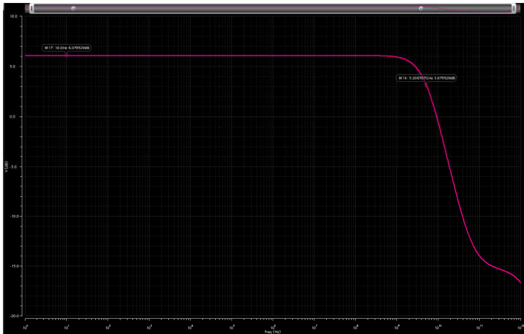
Fig. 3-21 Respuesta en frecuencia del OTA con W = 5.5 [\mu m] , R_L = 1300 [\Omega] , g_m = 1846.02 [\mu\Omega^{-1}] , A_{v-sim} = 6.0795 [dB] y BW_{sim} = 5.21 [GHz] .
