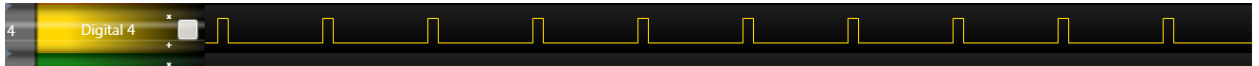
Figure 5-3, Signal used to Feed the machine, measured between PWML (JP2 pin 15) and GND.
