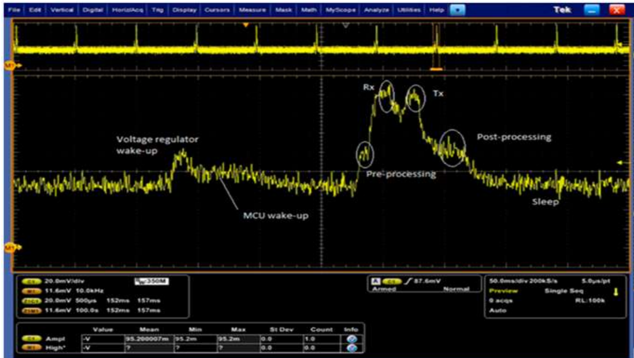
Fig. 3.12 Connection event waveform for Intel A-101. Figure taken from [Garcia-Espinosa-18].
