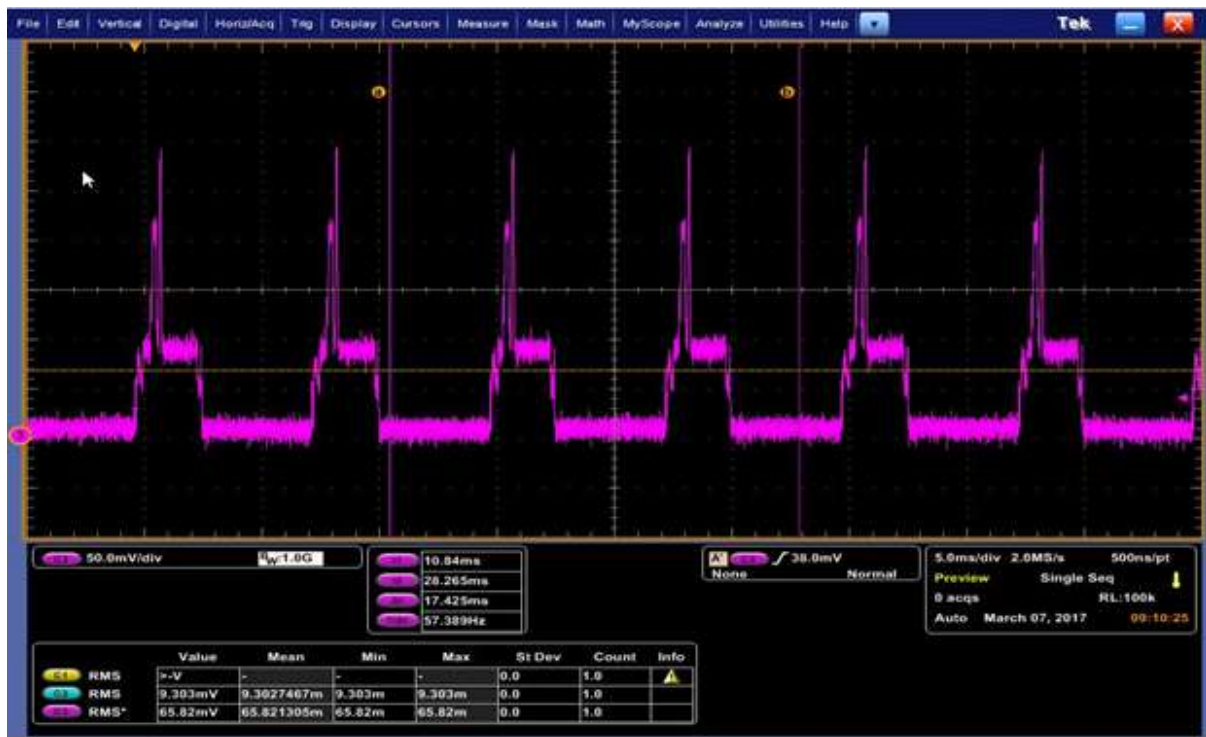
Fig. 3.7 BLE connection event when the connInterval is set to 7.5 ms.
