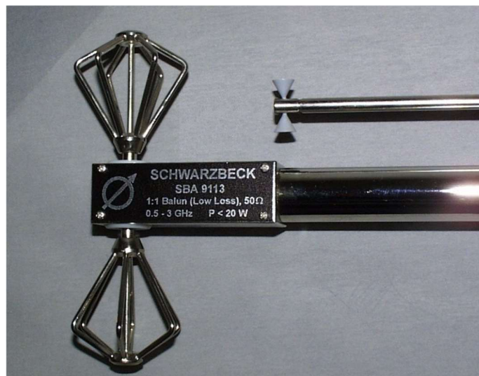
Figure 1-6 Examples of 3D biconical antennas. Taken from [22], CC license CC BY-SA 3.0.
