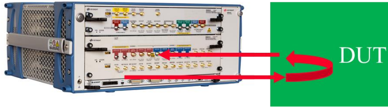
Fig. 1.16 JTOL setup showing BERT and loopback in DUT.
