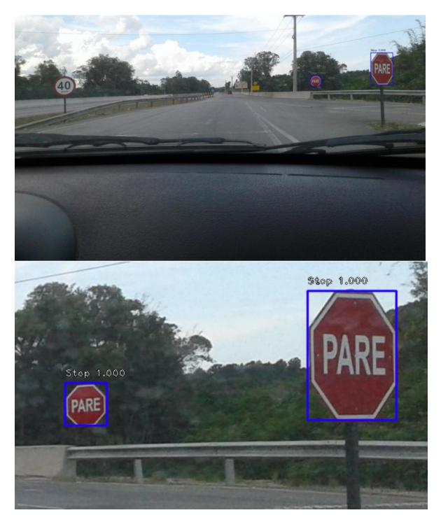
Figure 20: Detection and recognition of two Stop traffic signs within an image.
