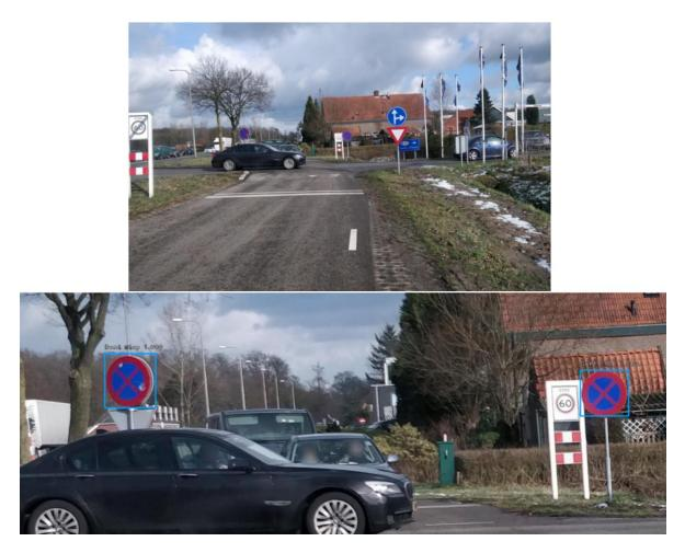
Figure 19: Detection and recognition of two Do not stop traffic signs within an image.
