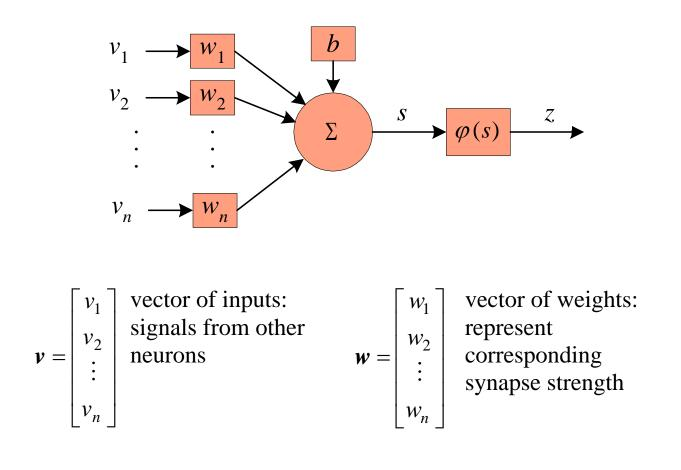
*b* is the bias or offset term  $s = b + \mathbf{v}^T \mathbf{w}$  is the activation signal  $z = \varphi(s)$  is the output signal
