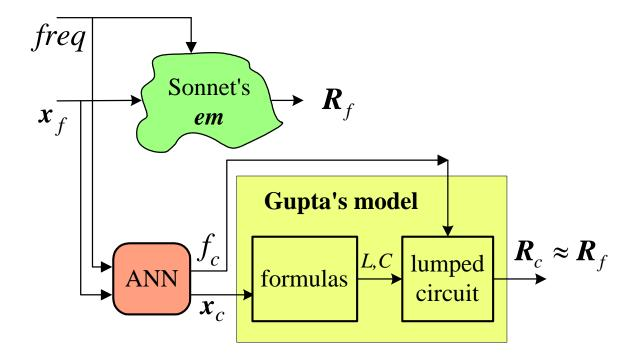
implementation: an OSA90/hope<sup>™</sup> child program simulates the coarse model at a different frequency variable through Datapipe
