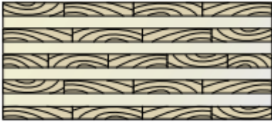
Figura 15: Capas de CLT ( (FP Innovations , 2013)
