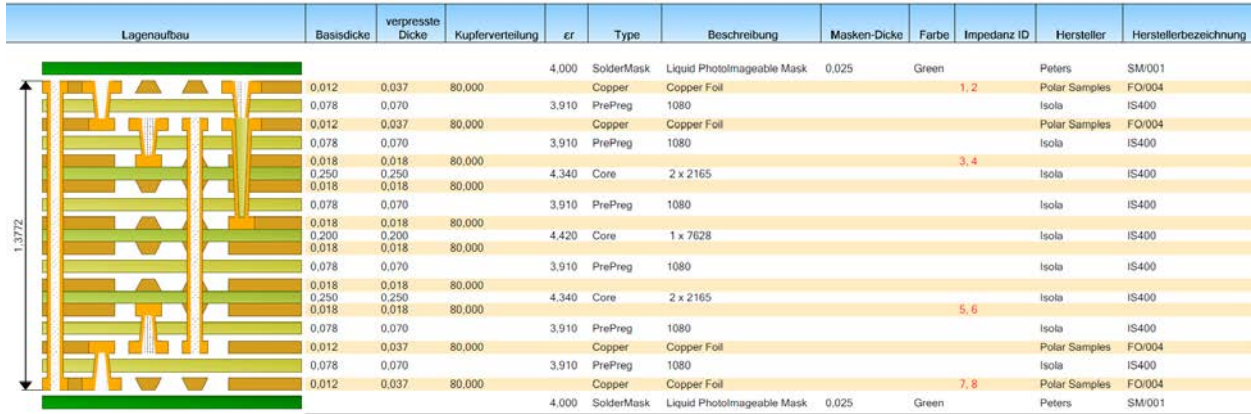
Fig. 4.7 Ten layers PCB stackup with HDI used in MiP. From [MOS-13]
