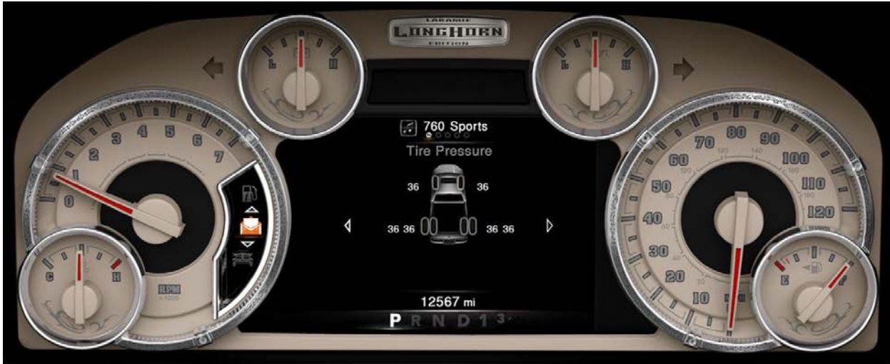
Fig. 2.16 Example of a full size automotive instrument cluster with mechanical and digital features. From [Gunaxin Media-17].
