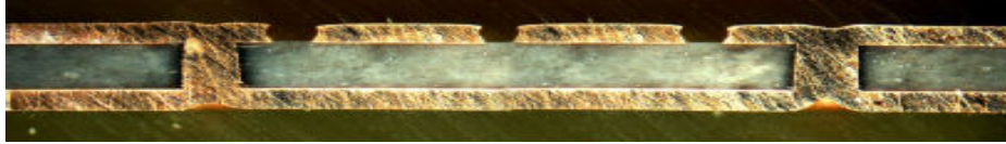
Fig. 1.8 Cross section photograph of the implemented transmission line.
