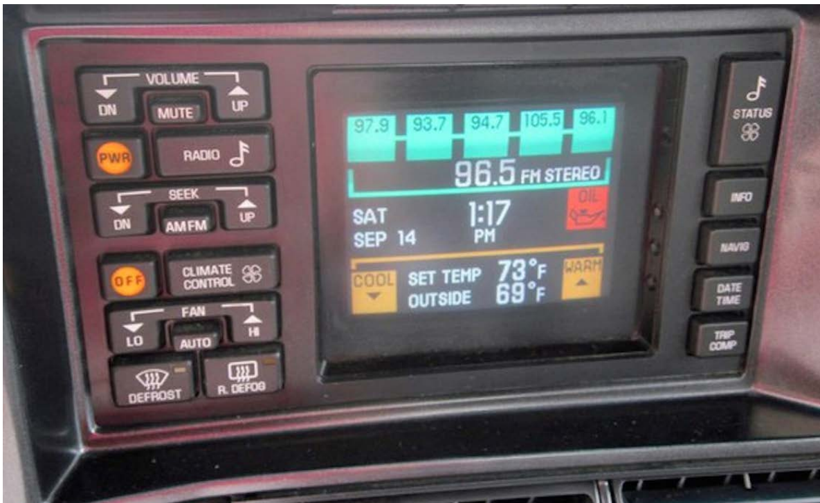
Fig. 2.1 Legacy automotive HMI: Touchscreen infotainment system from 1989 Oldsmobile Toronado Trofeo, called the Visual Information Center (VIC). The touchscreen was powered by a pair of 8-bit processors and gave the driver access to everything from the radio to engine management data. From [Business Insider-17].
