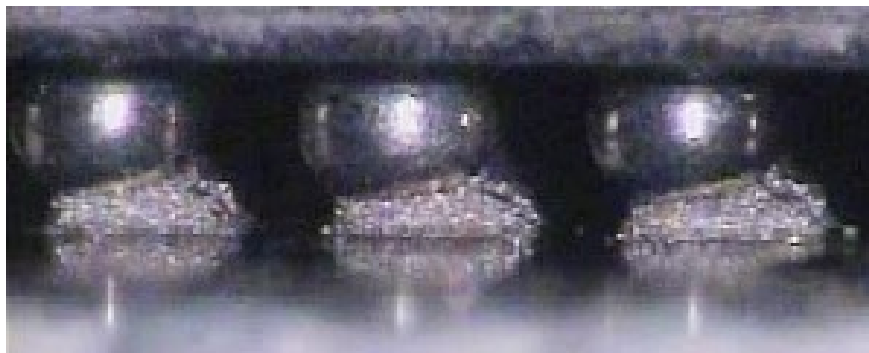
Fig. 3.17 Head-on-pillow phenomenon in BGAs. From [Indium-08]
