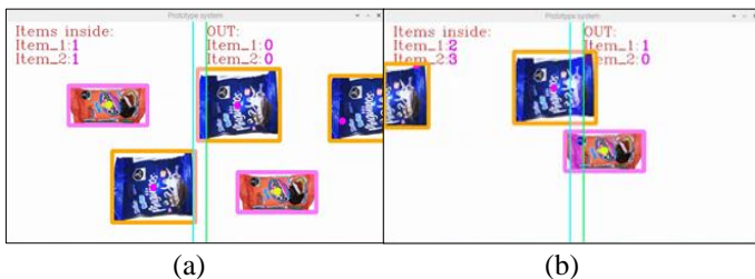
Fig. 10 Warehouse stock counting prototype running: (a) items entering to warehouse, (b) items leaving the warehouse.
