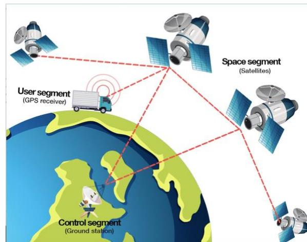
Figure 2: Global Positioning System.
