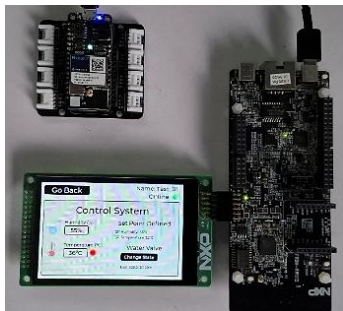
Fig. 15. Embedded application consuming web services from Particle IoT cloud REST API.
