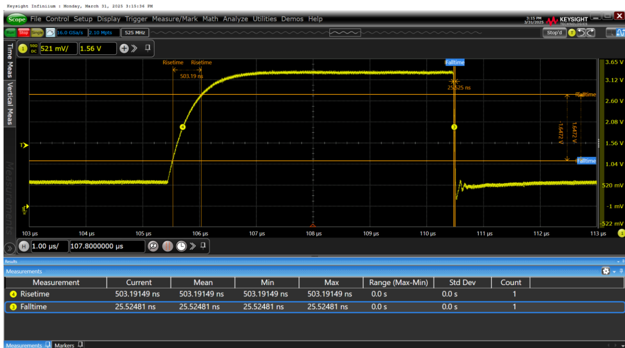
Fig. 3.6 Example of a 100kHz square signal, describing Rise Time and Fall Time measurements of the 20% to 80% swing voltage.
