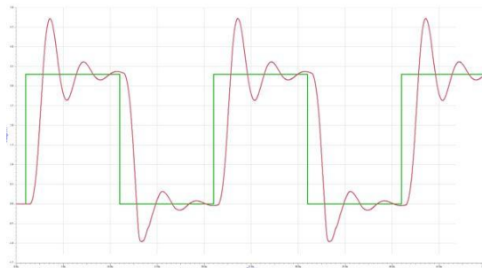
Fig. 2.2 Representation of an electrical signal and how accurately it represents its intended shape when sent through a channel. Figure taken from [16].
