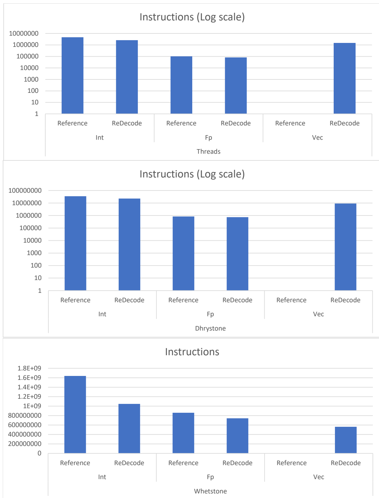
Fig. 5-2 AluAccess Comparison between the 3 benchmarks, each FU has a bar for each model, Threads and Dhrystone are on a logarithmic scale.
