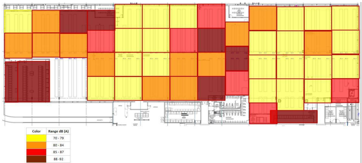
Figure 2 – Intel's Guadalajara Design Center validation lab Noise Level Mapping
