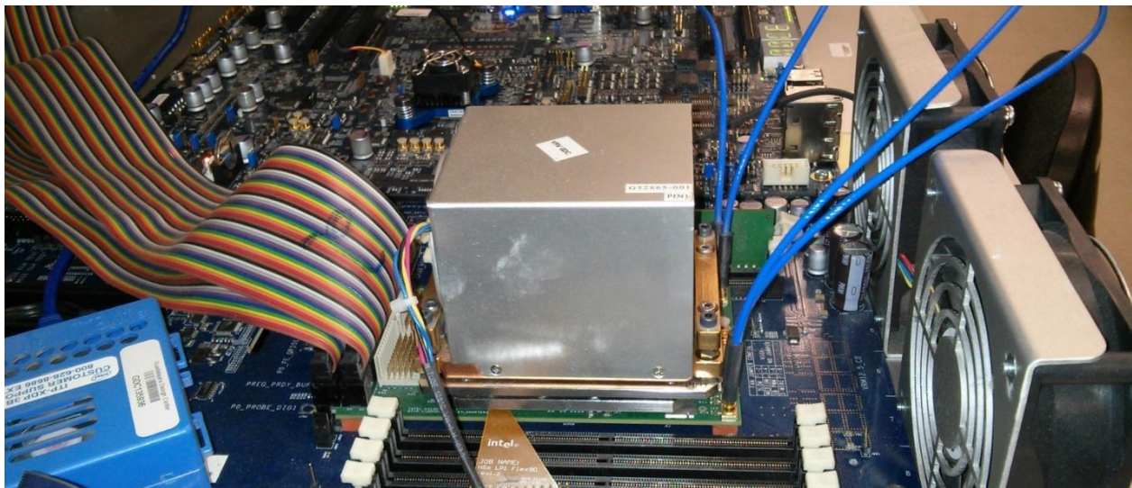
Figure 5 – Server CPU Heatsink solution example.
