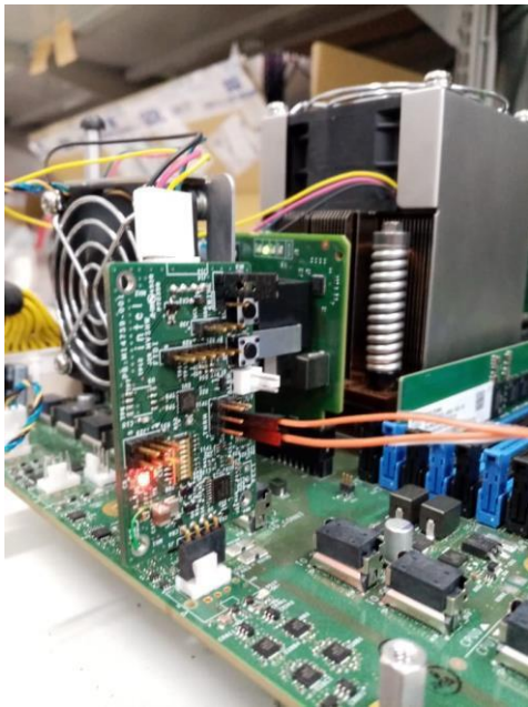
Figure 46- PFC Installed in a Server Validation Platform and an Electrical Validation Platform
