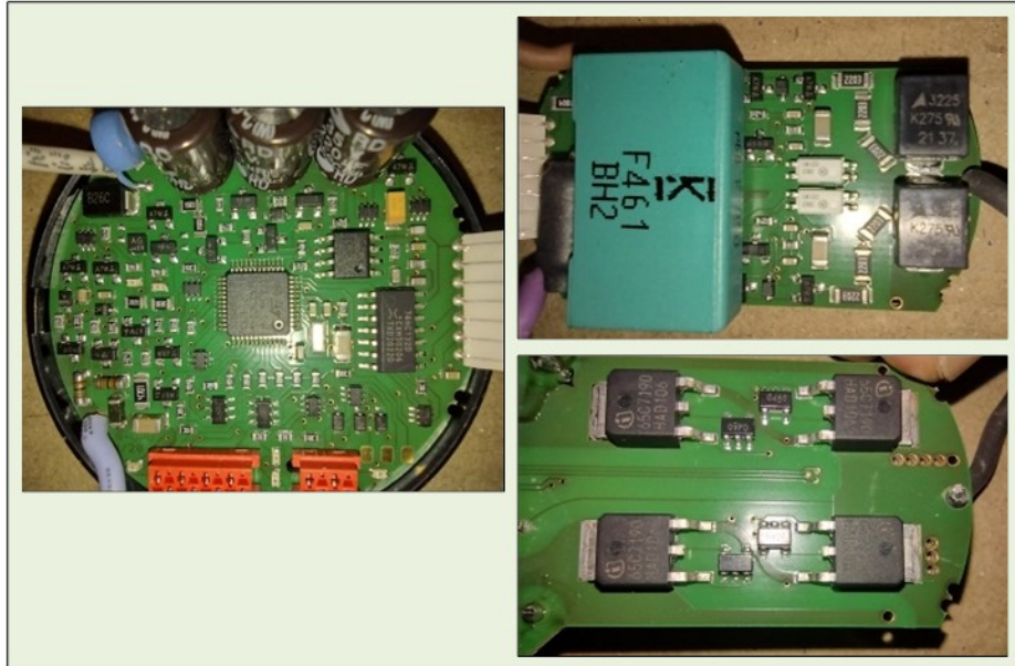
Fig. 0-3 LCNUPU Digital board (left) and Power output board – top side (upper right) & bottom side (lower right).
