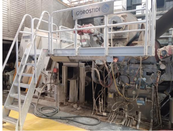
Fig. 2.1 Rodsizer-spooner section of a papermaking machine.
