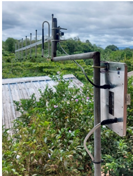
Figure 4. Transmitter used to validate propagation models of TV White Spaces (TVWS) technology for wireless broadband in rural Colombian rain forest [60]. (Photo courtesy of Prof. Andrés Navarro-Cadavid).
