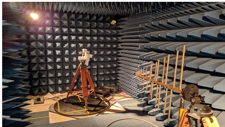
Figure 3. Setup for measurement of a magneto-dielectric antenna in an anechoic chamber at the Federal University of Campina Grande (UFCG), Brazil. (Photo courtesy of Prof. Glauco Fontgalland).
