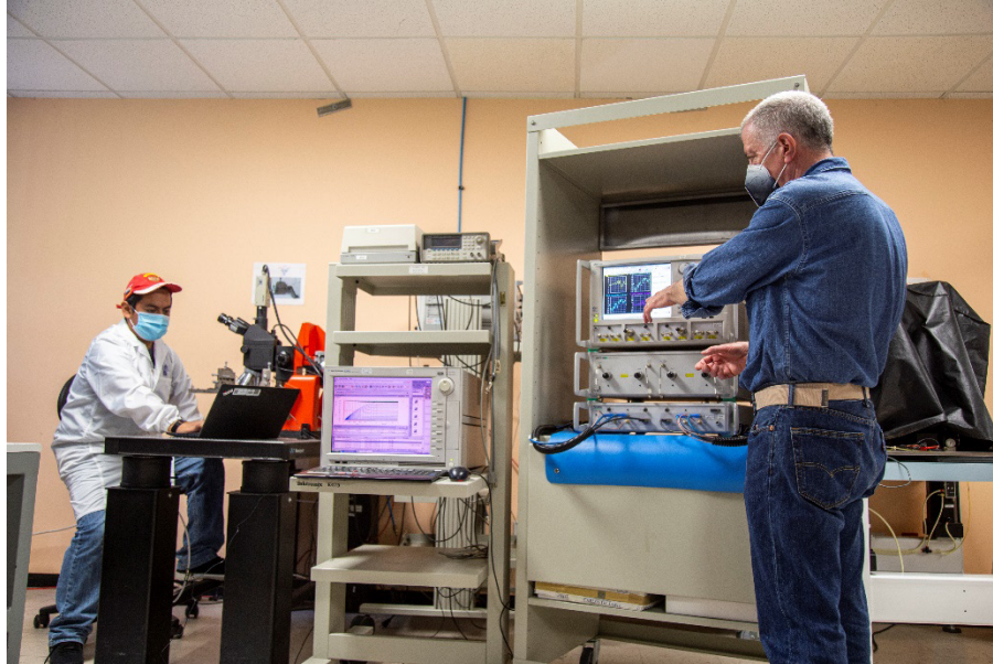
Figure 8. Advanced VNAs available at INAOE, in Puebla, Mexico: one capable of two-port measurements up to 67 GHz, and the other one able to perform four-port measurements in the 10 MHz to 70 GHz range, as well as two-port measurements up to 110 GHz. (Photo courtesy of Prof. Roberto S. Murphy).
