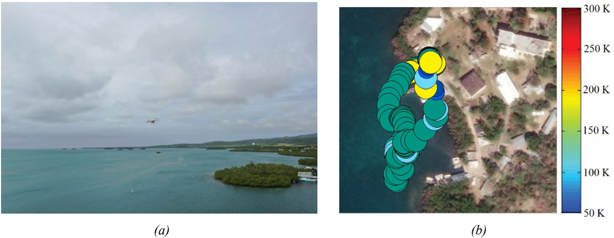
Figure 10. Microwave remote sensing in Puerto Rico: (a) UAV carrying microwave radiometer flying over Magueyes Island; (b) brightness temperature measured with radiometer during field campaign at Magueyes Island [125], the circle size represents the antenna footprint. (Photos courtesy of Prof. Raúl Rodríguez-Solis).
