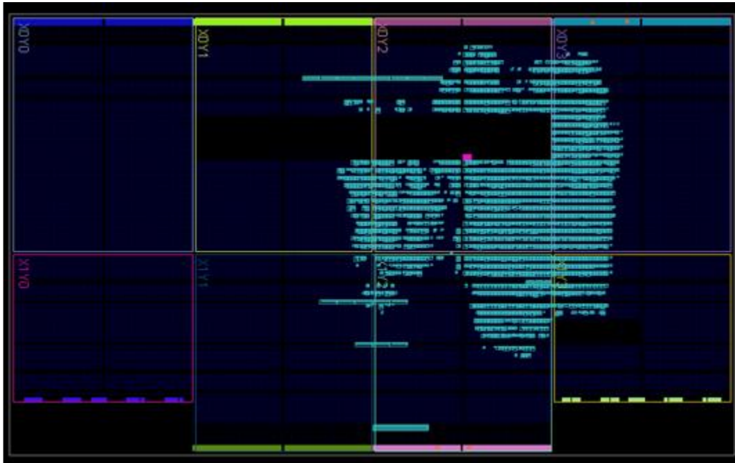
Figure 5-7 - FPGA routing resources of the SHA-3 512 Software Implementation on an xc7a100tcsq324-1 FPGA.
