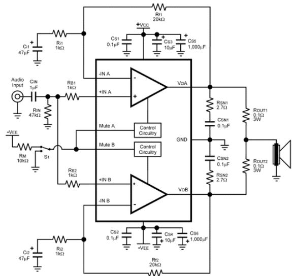
Figure 3-5 Operational Amplifier LM4780 Schematic
