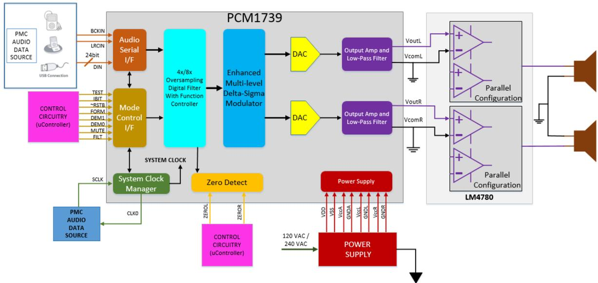
Figure 3-2 Proposed Block Diagram with commercial devices
