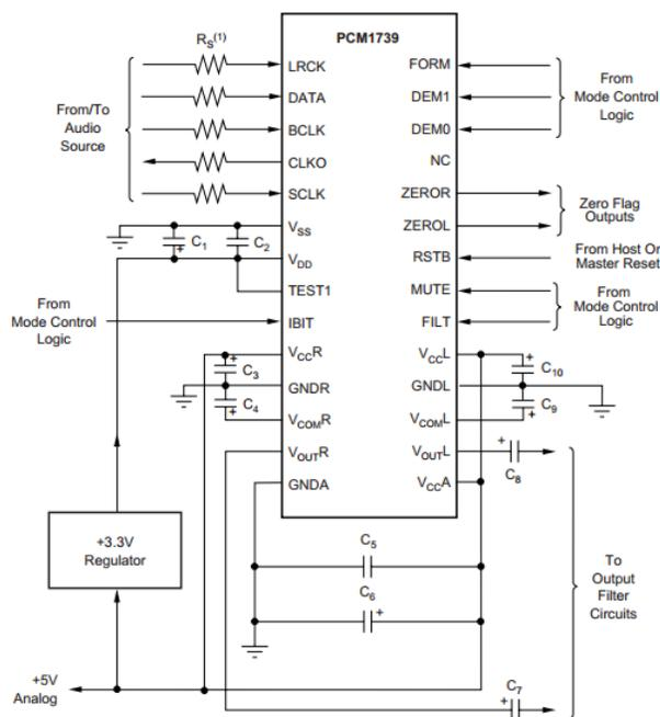
Figure 3-3 DAC PCM1739 Schematic
