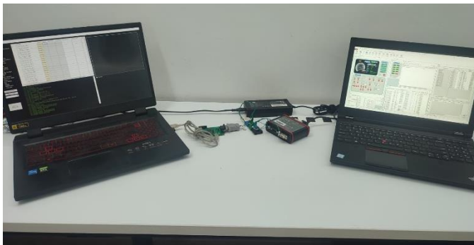
Fig. 3. USB-CAN interface in a CAN bus system
