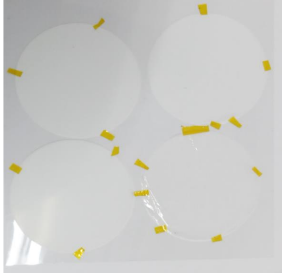
Fig. 2.3. Photo of nanopores polycarbonate (PCTE) membranes before metallization.
