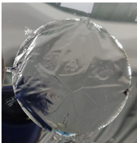
Fig. 2.6. Polycarbonate nano porous membrane metalized with silver (500 nm of Ag) photo.
