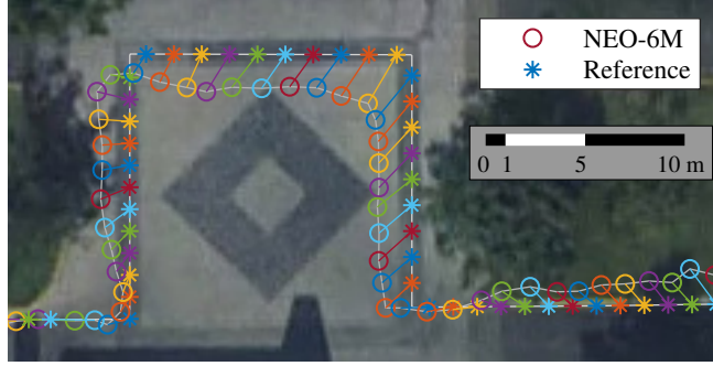
Fig. 3.2. Synchronization of the low-cost GPS receiver with respect to the reference path, based on the change in direction of the user and recognizable landmarks in the orthophoto (only a close-up section of the image is shown for clarity).
