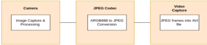
Fig. 6. JPEG Coding flow diagram
